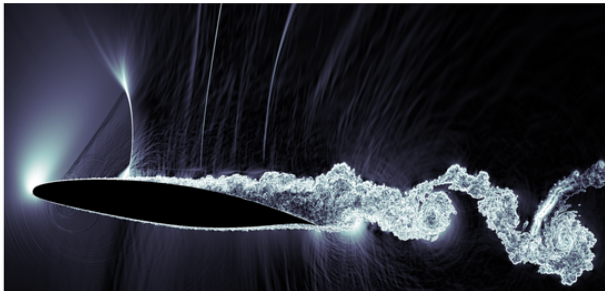
Figure 1: Numerical Schlieren snapshot of fully developed buffet flow at M = 0.7 , Re = 6 \times 10^5 , and \alpha = 7^\circ .
